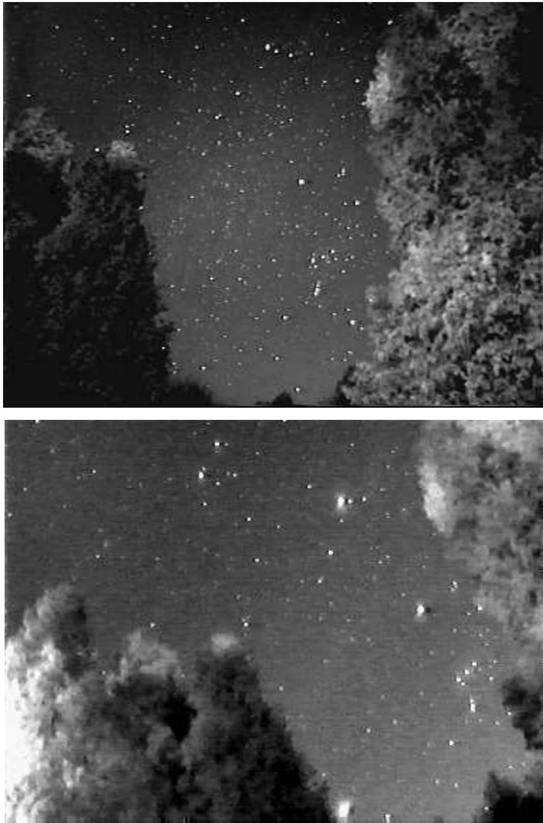
Figure 4 – Example of images for long exposures. Top: COMPUTAR f/1.2 , f = 4 mm. The best lens in the tests. Bottom: COMPUTAR f/0.8 , f = 3.8 mm. The fastest lens in the tests. These images have been enlarged so that the pixels are visible, to allow a critical appraisal of the quality.
